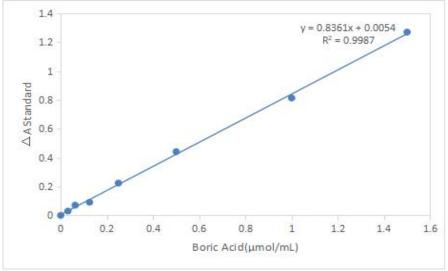
Figure1. Boric acid standard curve Examples:
